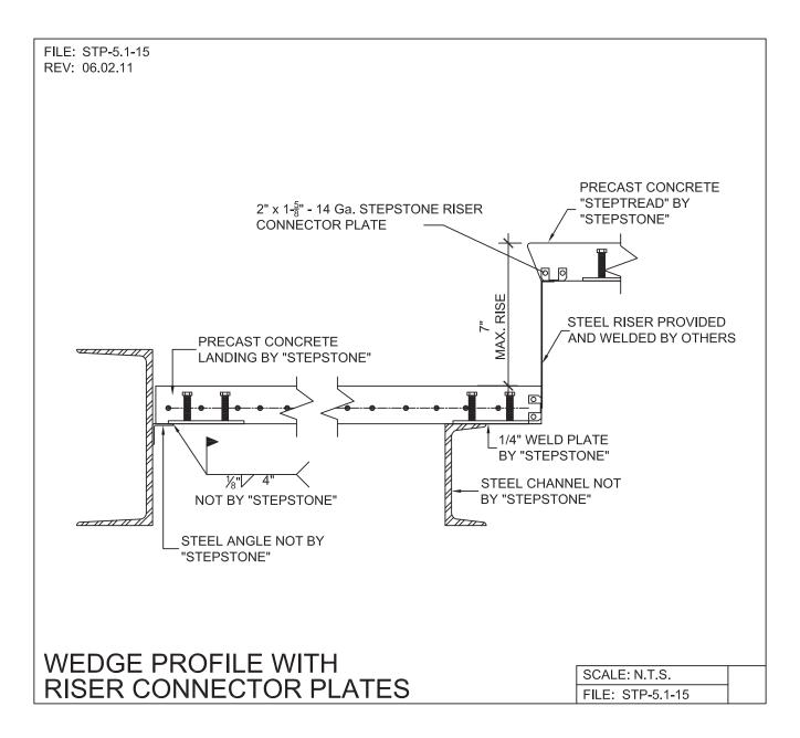
PRECAST CONCRETE TREADS AND LANDINGS SHOWN ON PLANS SHALL BE FROM THE LONG SPAN "STEPTREAD" SYSTEM BY "STEPSTONE, INC." OF GARDENA, CA FOR STEEL CONSTRUCTION. THE MANUFACTURER IS TO SUPPLY ALL PRECAST CONCRETE "STEPTREAD" SYSTEM PARTS, FEATURING BOTTOM WELD PLATES FOR WELD-ON CONNECTIONS. ALL REINFORCING AND CONNECTION PLATES WILL BE ZINC PLATED. ONLY ITEMS NOTED AS BY "STEPSTONE, INC." WILL BE FURNISHED BY "STEPSTONE, INC." SUCH ITEMS ARE TO BE INSTALLED BY OTHERS.
